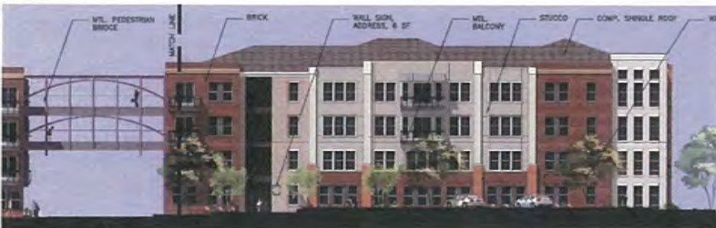
06 Elevation - River Fern Drive (East) Scale: 1/16" = 1'-0"
