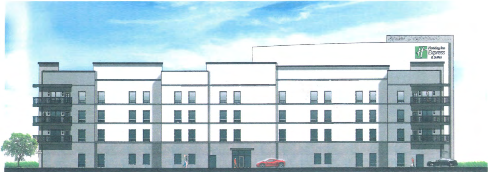
SOUTH ELEVATION/65.5% stucco and 34.5% porcelain tile
