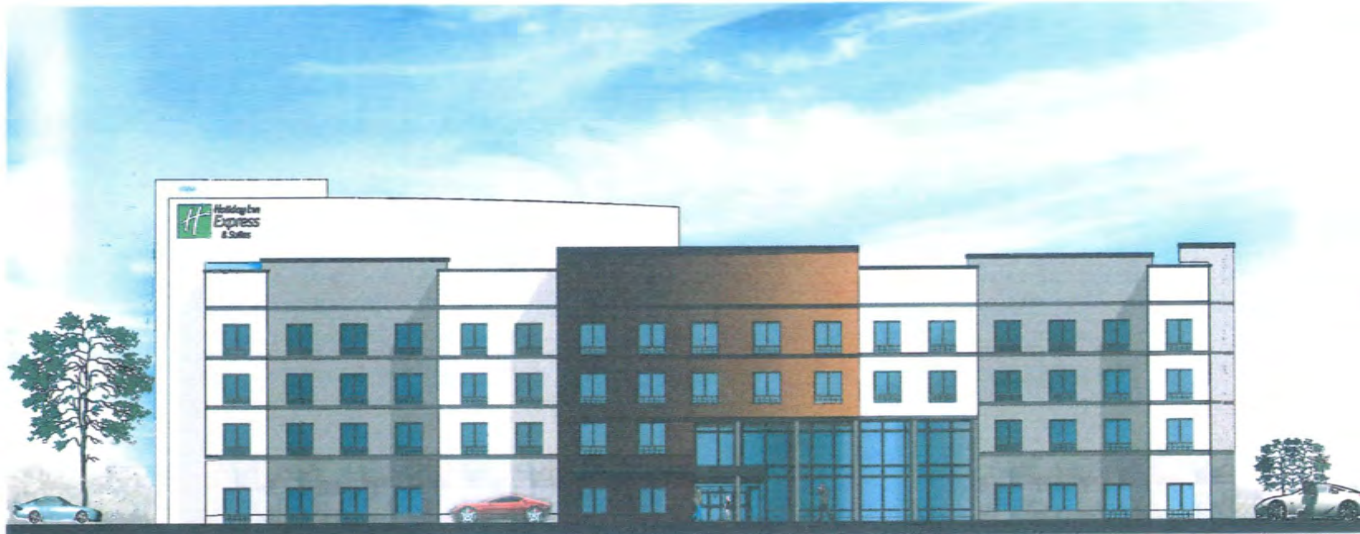
NORTH ELEVATION/83.8% stucco and 16.2% porcelain tile
