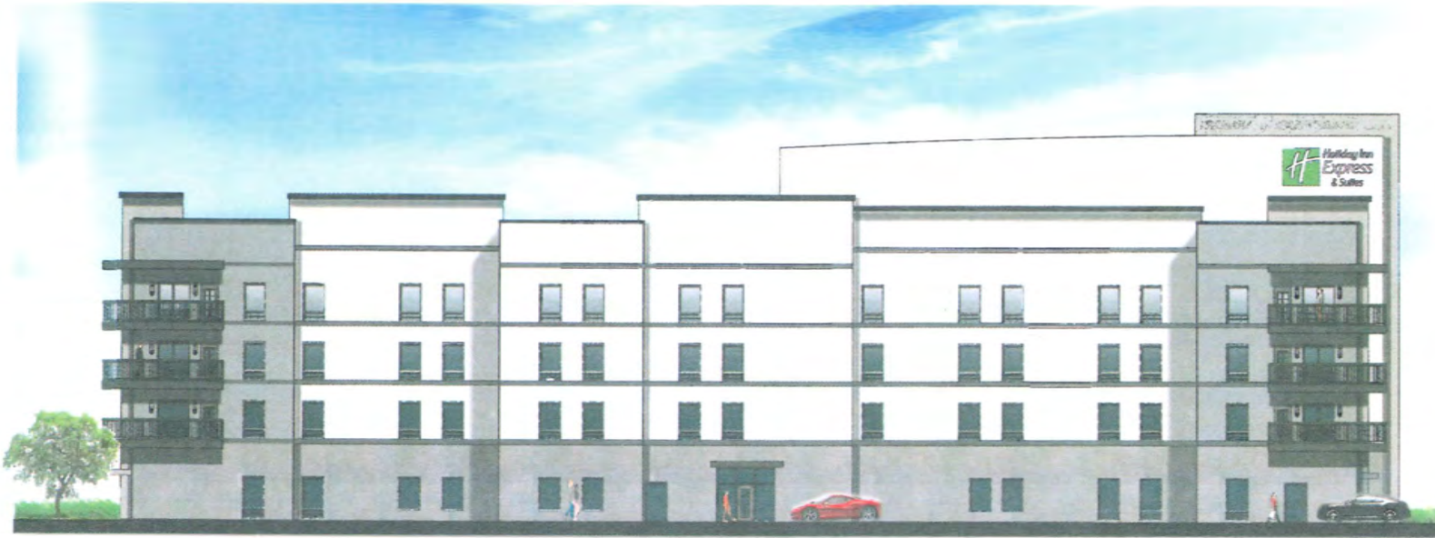
SOUTH ELEVATION/65.5% stucco and 34.5% porcelain tile
