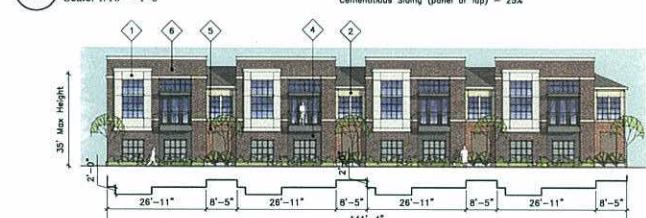
16 Building IX Front Elevation Scale: 1/16" = 1'-0"
