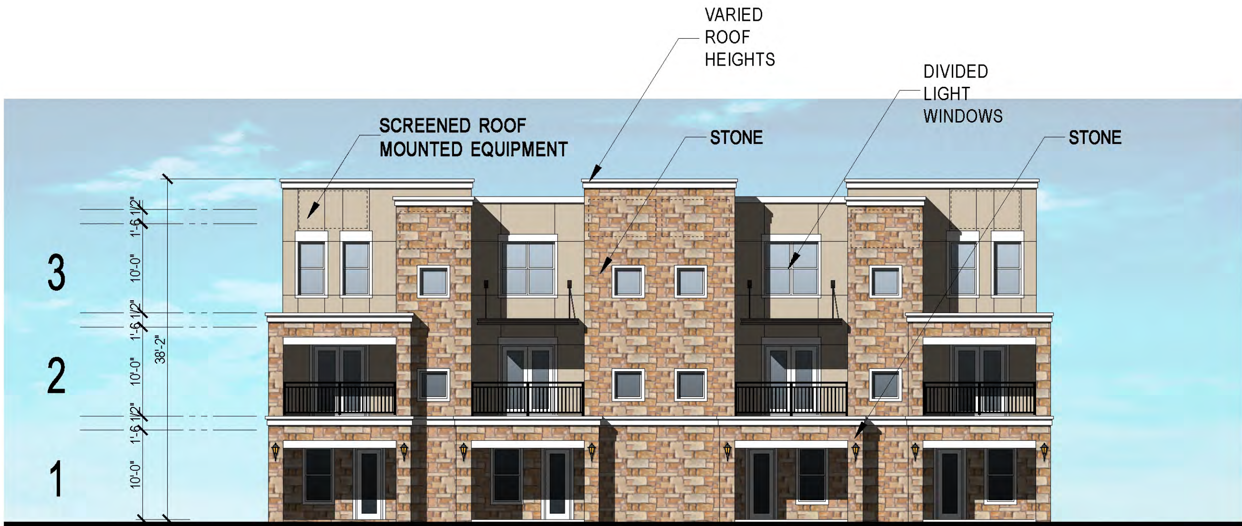
FRONT ELEVATION (POOL SIDE) BUILDING TYPE VI STONE 66% STUCCO 34%
