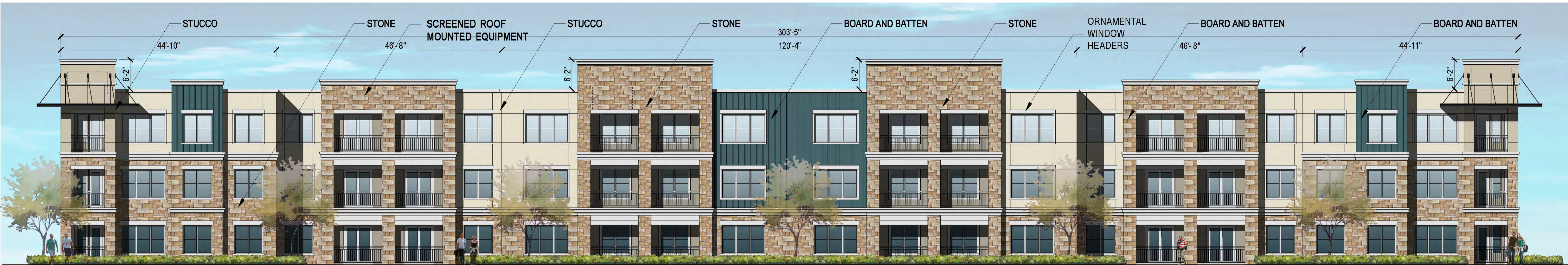
STREET ELEVATION (4' DEPTH ARTICULATION 69%) BUILDING TYPE IV
