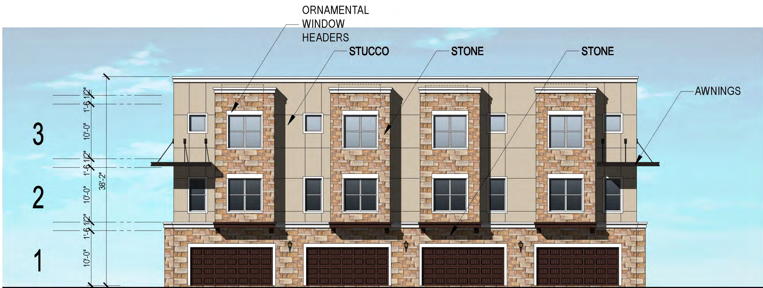
REAR ELEVATION (DRIVEWAY SIDE) BUILDING TYPE VI STONE 52% STUCCO 48%
