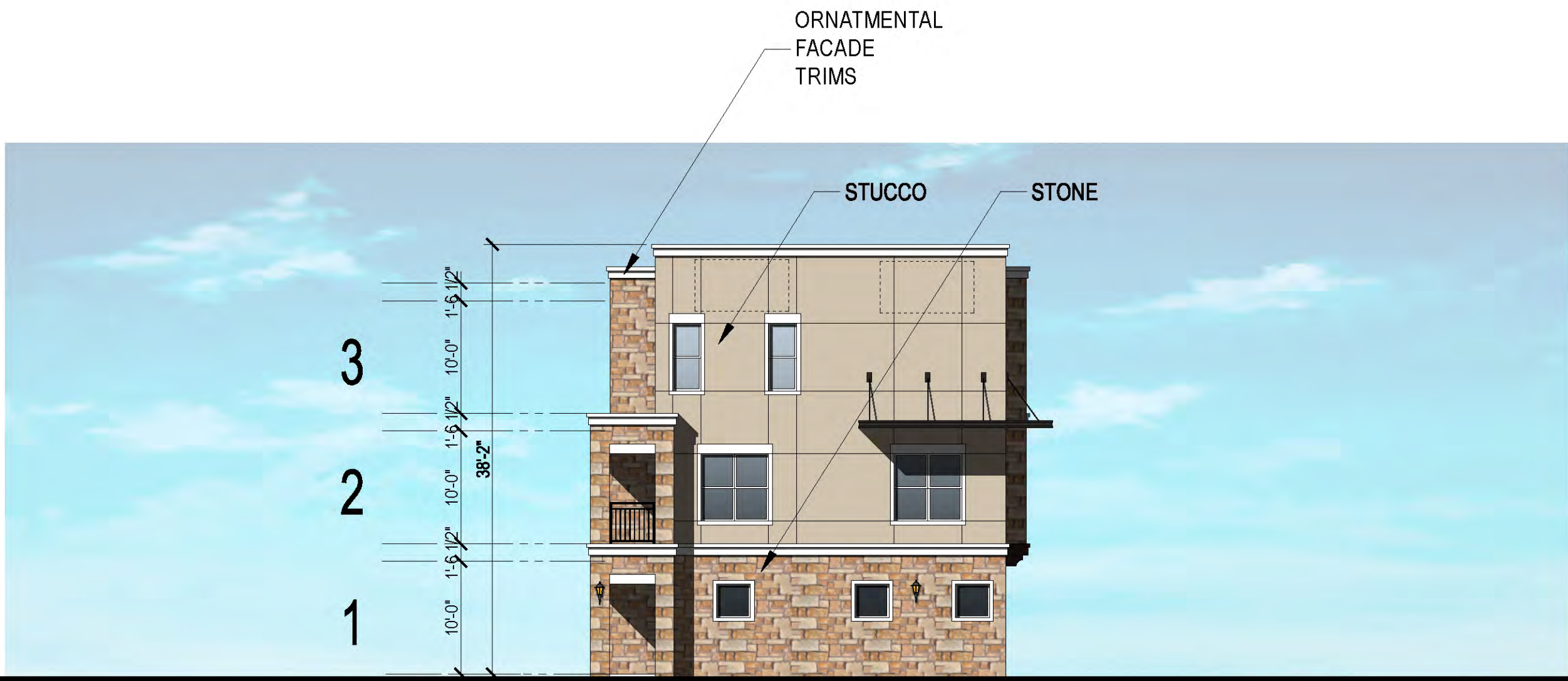
SIDE ELEVATION BUILDING TYPE VI STONE 45% STUCCO 58%
