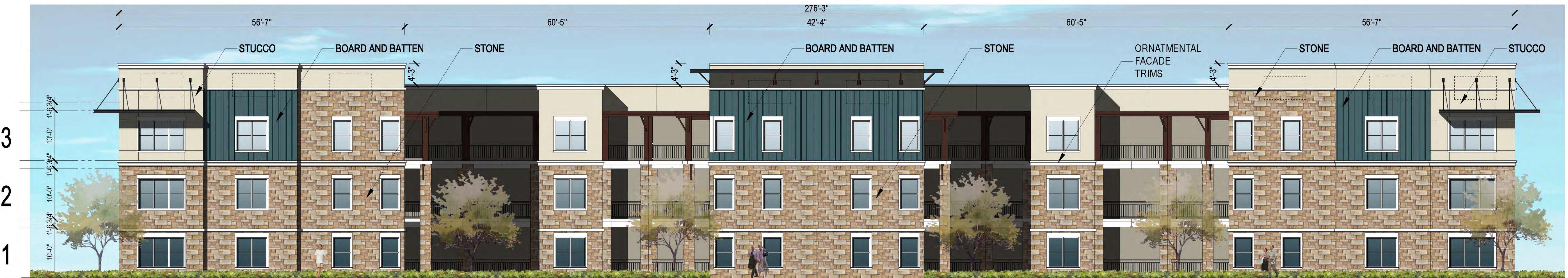
STREET ELEVATION (4' DEPTH ARTICULATION 43%) BUILDING TYPE II
